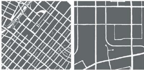
A figure ground study of downtown Los Angeles (left) and Irvine California (right) shows how the proportions of city blocks affect walkability.
